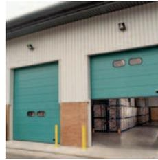
This type of door features ease of operation, weather resistance and versatility. Requirements for thermal insulation, maximum vision, ventilation with security and elegance can all be met. These doors can be manually operated by pull down rope or geared
