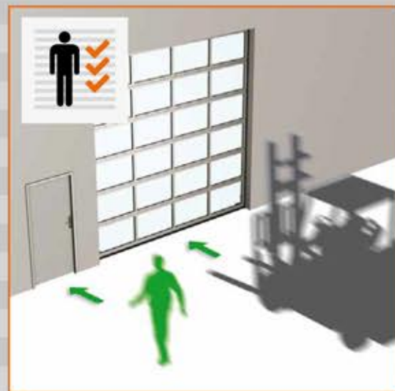
Completely separate doors for pedestrians and goods.
