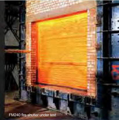
FM240 fire shutter under test
